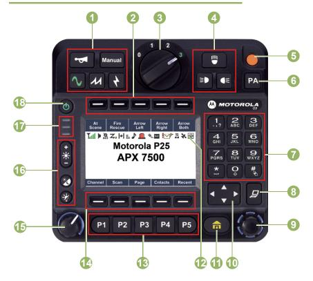
Siren Control Buttons Programmable Buttons (Top) **Response Selector Directional Buttons** Orange Button Public Address Button 6 Keypad Data Feature Button Mode Knob 4-Way Navigation Button Home Button Satus Icons Programmable Buttons (Bottom) Menu Select Buttons 15 Volume Knob **Display Backlight Control Buttons** LED Indicators Power On/Off Button
