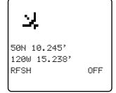
3 Press •, ••, or • directly below RFSH to obtain a new location fix. The top line will temporarily display PLEASE WAIT while the new location is being determined.
