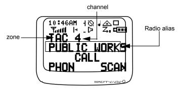
This figure is typical of what you see on your radio. The 64 x 96 pixel liquid crystal display (LCD) shows radio status, text, and menu entries.
