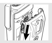
2 Pull the top of the battery away from the radio.
